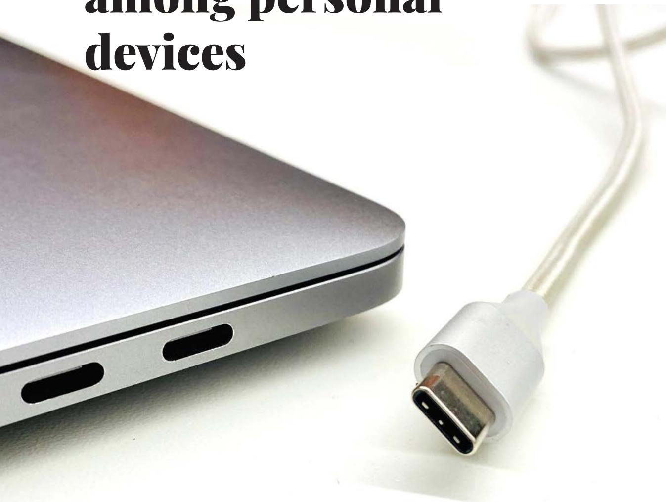
Designers can plan confidently around USB-C Power Delivery (PD) as the cross-platform standard. USB-IF now certifies PD 3.1 “Extended Power Range” up to 240 W, enabling high-wattage laptop charging from a single USB-C port—so long as the cable and charger are rated appropriately (E-marked 5 A cables for >100 W).<sup>10</sup> Generally speaking, most laptops will charge between 60-100W.
