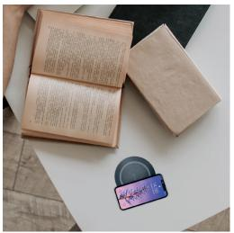
The ARC-H (LD) sub-surface wireless charger offers the ultimate in charging convenience. Designed with a charging range of .78-1.18" (20-30mm), ARC-H (LD) can be installed without the need to cut into work surfaces.
