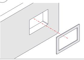
Connect GST cable to QF15 TUF HP module and place into cutout
