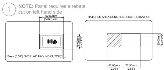
Example is representative of a 1.5mm (.06") thick mounting plate. Adjust rebate as needed to maintain 4mm (.16") rebate surface thickness if plate thickness varies.
