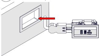
4 Clip right hand side of QF15 TUF HP module into cutout
