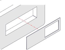
Connect GST cable to QF15 TUF HP module and place into cutout
