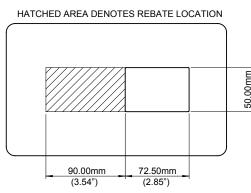
Example is representative of a 1.5mm (.06") thick mounting plate. Adjust rebate as needed to maintain 4mm (.16") rebate surface thickness if plate thickness varies.
