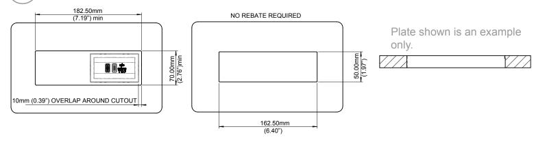
$\left(\begin{array}{c}2\end{array}\right)$  Fix plate to surface using adhesive
