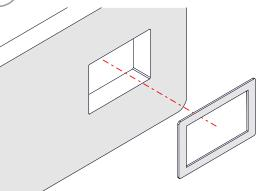
Connect right angled GST to QF15 TUF HP module and place into cutout
