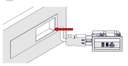
4 Clip right hand side of QF15 TUF HP module into cutout
