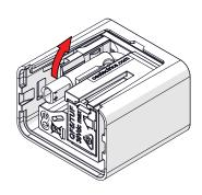
Slide GST08 cable through cable exit in Piccolo back
