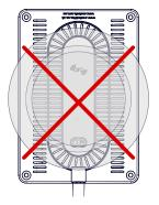
Pad misaligned - WILL NOT WORK The alignment guide must be used to guarantee accuracy
