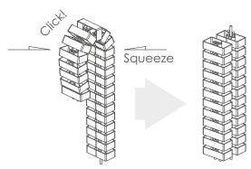
Determine required length. Roll Chain Links over itself and squeeze together. Chains links will separate.
