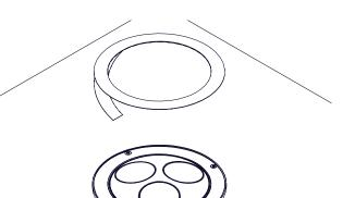
To fit the outer inlay, remove the VHB cover, align with the outer grommet, and then press down firmly.
