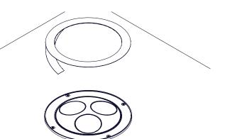
To fit the outer inlay, remove the VHB cover, align with the outer grommet, and then press down firmly.
