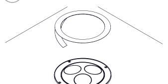
To fit the outer inlay, remove the VHB cover, align with the outer grommet, and then press down firmly.
