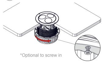
Peel back tape cover and press firmly
