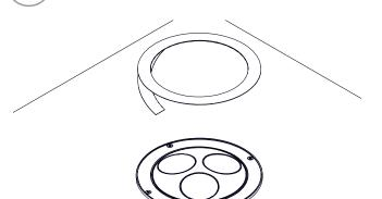
To fit the outer inlay, remove the VHB cover, align with the outer grommet, and then press down firmly.
