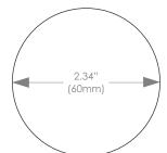
PIP can be installed into an industry standard 2.34" (60mm) grommet hole.
