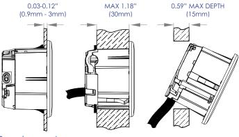
Snap-in mount Clamp mount Side exit cable mount
