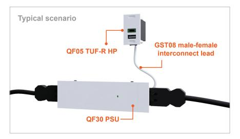
GST08 male to female leads are required to interconnect our ANIMATE system DC power products such as the TUF-HP 72W USB charger, QF30 PSU (Power Supply Unit) and QIKPAC battery. Leads are available in 0.5m, 1m, 1.5m and 2m lengths. Leads must be correctly aligned to slot together easily, do not force connectors together.
