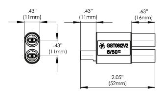
Align + and - symbols on the adapter to the text on the male and female connectors. **Do not force** connectors together.
