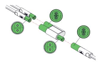
GST08 2-way adapter connections can be locked and secured to surfaces using a GST08 Cable Retention Clip.
